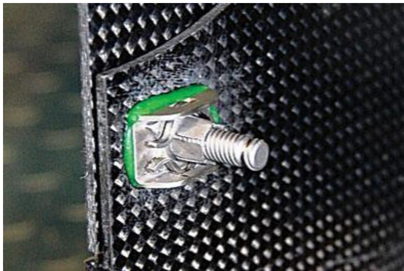
The FC43 structural panel fastener prevents delamination in composites (Aerospace)
