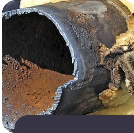
Corrosion and delamination to grow between the insulation and the pipeline surface
